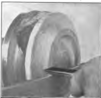
Fig. 127. Scraping with Chisel.
